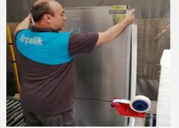
Figure 5: Applying the protector to the refrigerator
